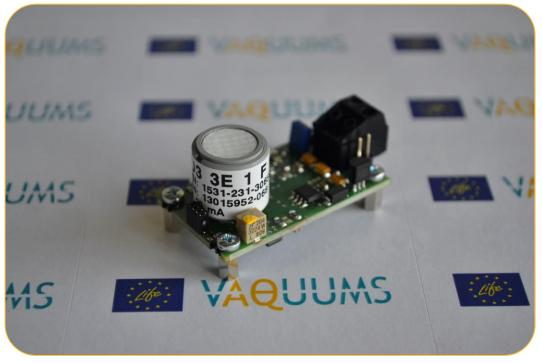
The Citytech O3 3E1F is an electrochemical ozone sensor. According to the manufacturer it can measure concentrations between 0 and 1 ppm, with a resolution of 0.03 ppm. It is mostly used for industrial applications.
